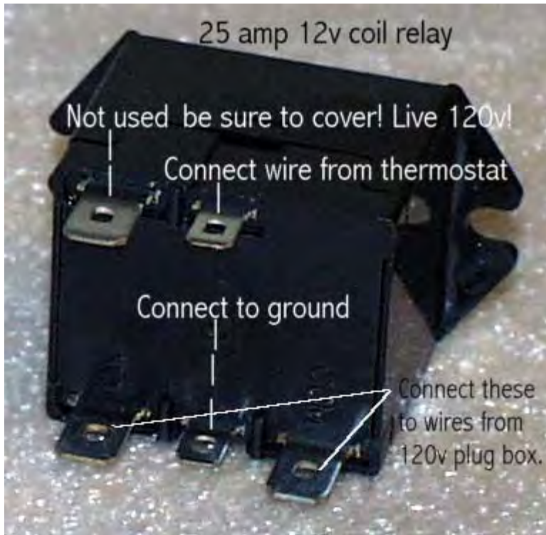
Here is the "heart" of the system--the 25 amp relay.
